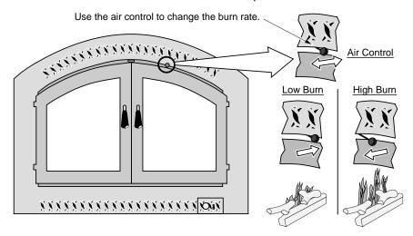
Warning: The air control becomes hot during operation - use gloves or a tool to prevent burns.
